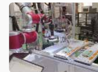
Screwing operations on lamp assembly
