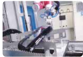
Dust removal from lighting covers
