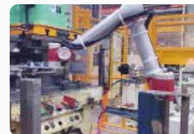
Machine tending for exhaust systems
